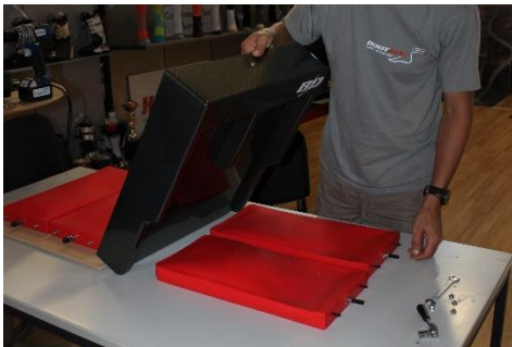
After the pump supply line is disconnected and all mounting hardware is removed it is then possible to remove the old pillows.
