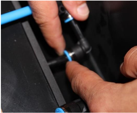
By pressing against the blue ring, the connection of the pump supply line and the BD PILLOW VAC III is separated.
